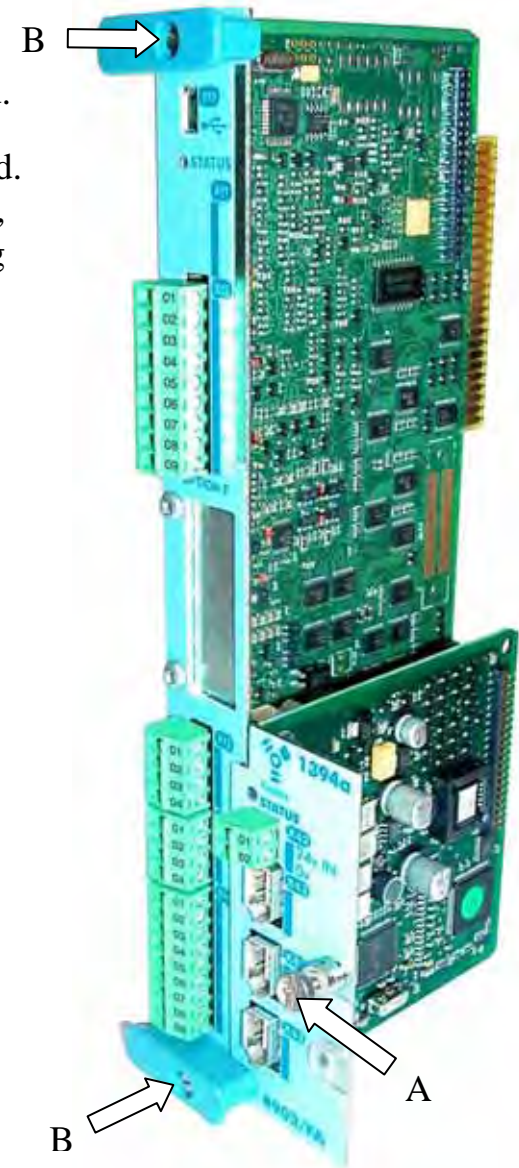
Figure 2 Control board with an Option Card correctly mounted
