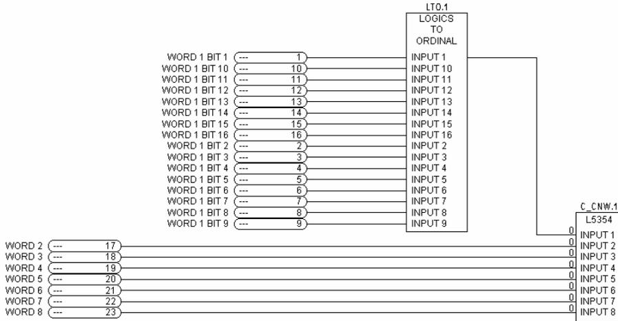
Figure 6. Logical to Ordinal and Value LINK Setup
