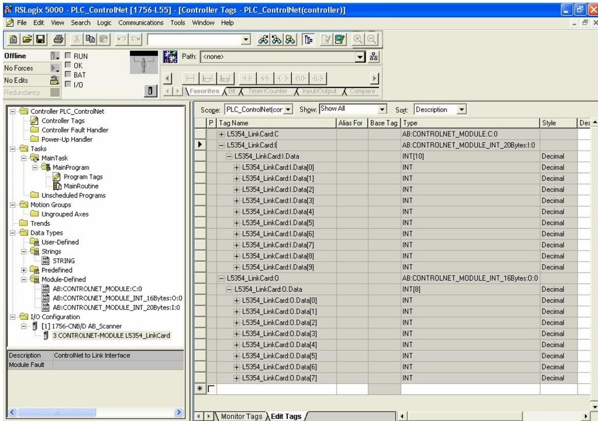
Figure 14 ControlNet Data allocations for the PLC
