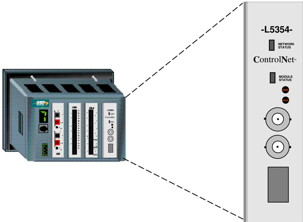
Figure 1. L5392 LinkStation with L5354 ControlNet LinkCard
