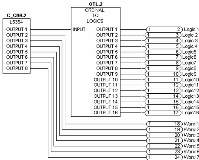
Figure 7. Ordinal to Logical and Value LINK Setup
