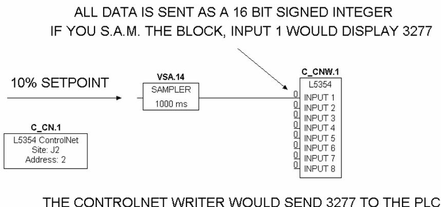
**Figure 5. Basic LINK Setup**
