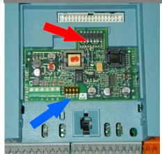
The Speed Feedback Card is required only for closed loop Flux Vector Control
