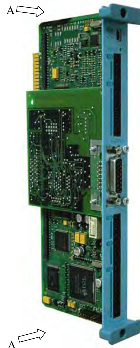
Figure 2 Control board with an Option Card correctly mounted
