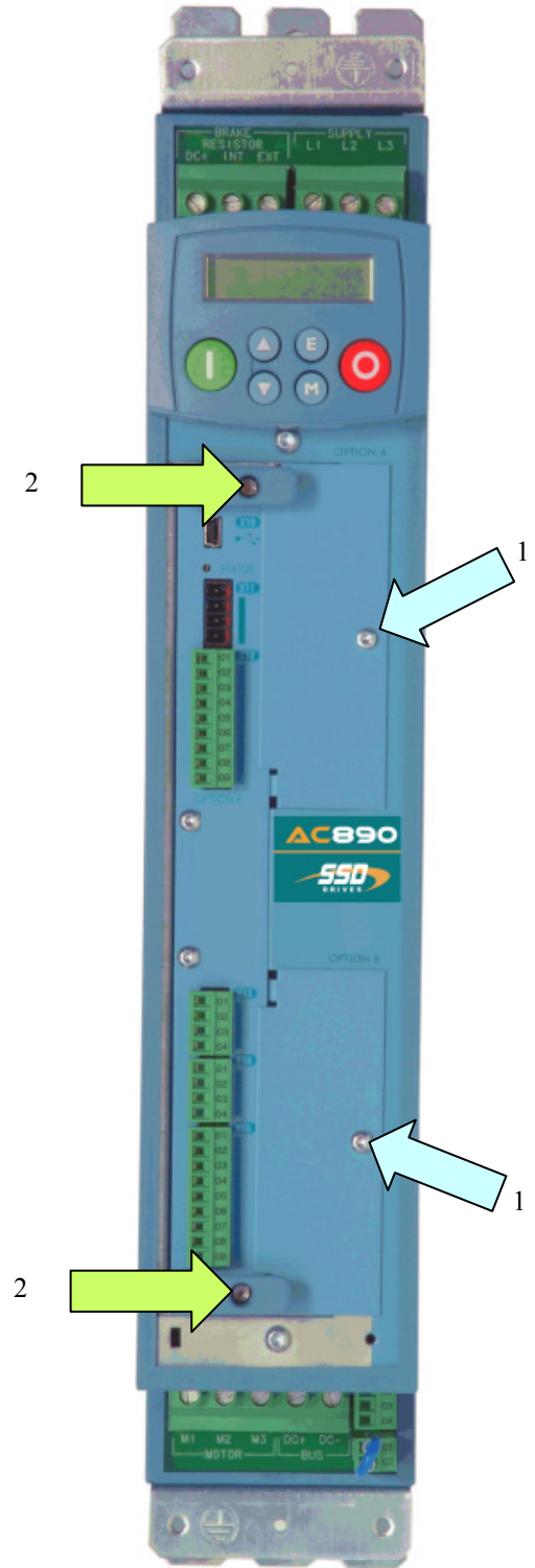
Figure 3. Front of 890 drive showing Control Board fitted
