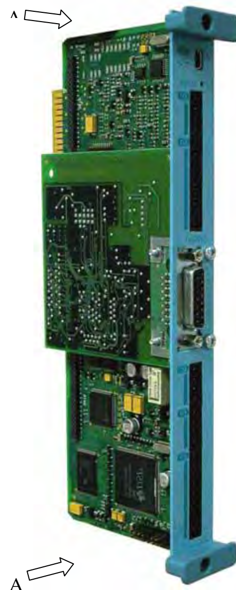
Figure A-1 Control board with an Option Card correctly mounted
